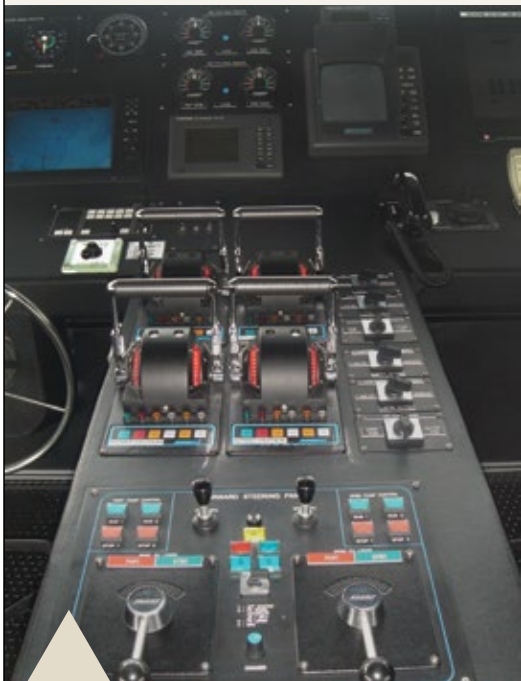
A 4-engine electronic propulsion control with Kobelt steering gear and rudder angle indicators. The complete package is provided by Kobelt.
